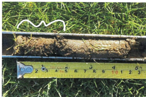
Photo 6: A thick thatch layer impedes infiltration of surface water
